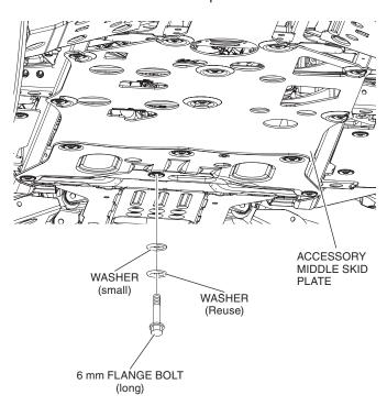
8. Tighten the loosely installed hardware to the values specified in the Torque Chart.
